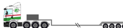
4-axle towing truck + 4-axle lowbed trailer, swing axle – 12 t/22 t; twistlock, removable gooseneck
