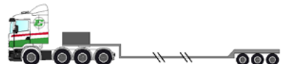
4-axle towing truck + 3-axle lowbed trailer, swing axle – 12 t/22 t; twistlock, removable gooseneck
