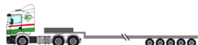
3-axle towing truck + 4-axle our 5-axle MEGA SEMI trailer; extendable, ramps, widenings, twistlock
