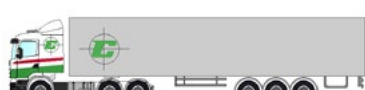
2-axle/3-axle towing truck + 3-axle MEGA trailer of expandable width; 7.0 t / 1 m; JOLODA-rails-systems; ramps
