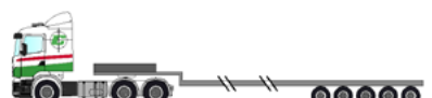
3-axle towing truck + 5-axle double extendable SEMI trailer, hydraulically steerable, ramps, widenings
