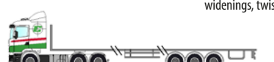
3-axle towing truck + 3-axle MEGA platform of double extendable, hydraulically steerable, ramps, widenings, twist
